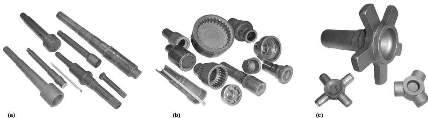
Fig. 2 Parts made by (a) forward extrusion, (b) backward extrusion, and (c) lateral extrusion. Courtesy of Metaldyne Corporation
